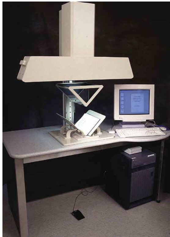
Figure 1. The PARC BookScanner, designed to scan rare and fragile books at 300 ppi 8-bit greyscale or 24-bit color. The book is opened to only 90° and placed, facing up, in the cradle; the two-paned glass ‘wedge platen’ descends to press both left & right pages flat simultaneously, while also pulling the camera assembly down to ensure precise geometry. Special DIA processing is required to enhance image quality due to many constraints on illumination & optics.
