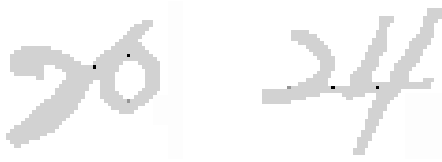
Figure 9. Segmentation points located by the NN-based approach
