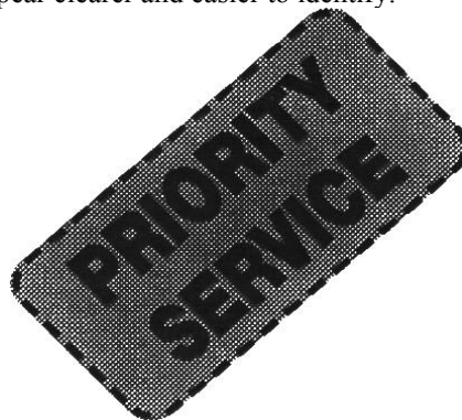
Figure 1. This child image has been mapped to original gray scale image by partial thresholding (if pixel value P(x,y) \leq T1 , keep original value, otherwise P(x,y)=255 )
